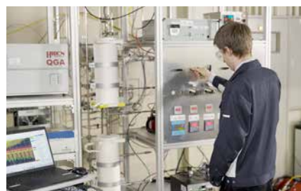
Bench plant for syngas production from NH 3 and CO 2
