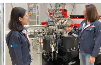
Secondary ion mass spectrometry with high mass and spatial resolution (NanoSIMS)
