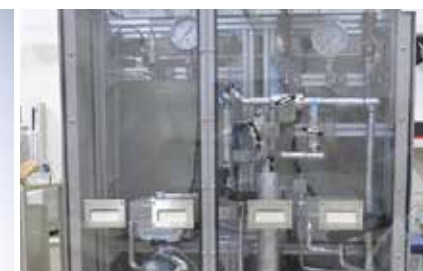
High-pressure hydrogen generator
